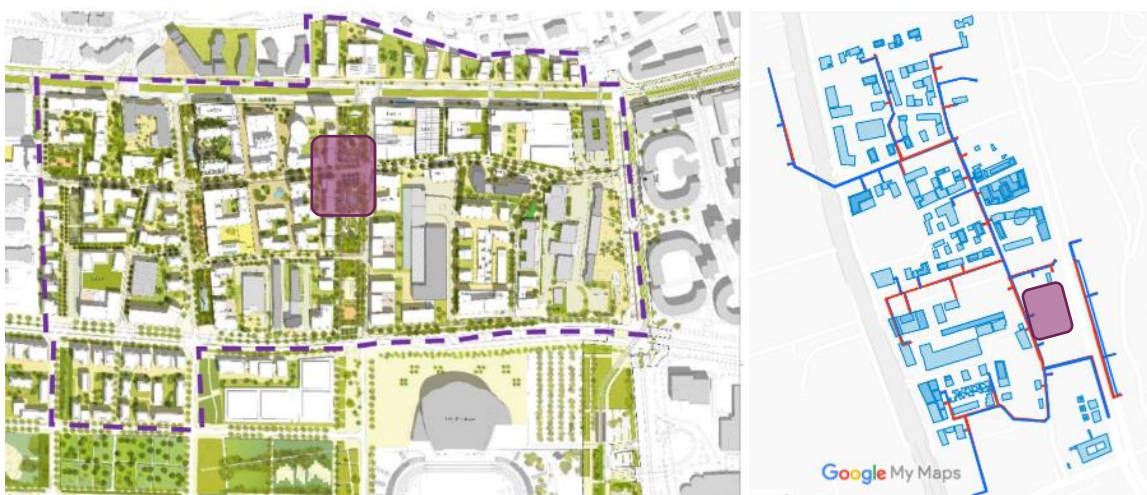
Figure 47 : left - in violet, the perimeter of the DHCN operation under the PDS contract – IMREDD and NEXITY buildings are highlighted under the red rectangle in the centre upper area (Source: EPA Plain du Var, addition by EDF); Right - planned DHCN layout and overlay of existing buildings ( source: https://www.google.com/maps/d/viewer?mid=1TkVPt5Z4ZqCFmPZZu81-RcsMxyv98VwH&ll=43.680735227580634%2C7.2003187737274175&z=16 )
