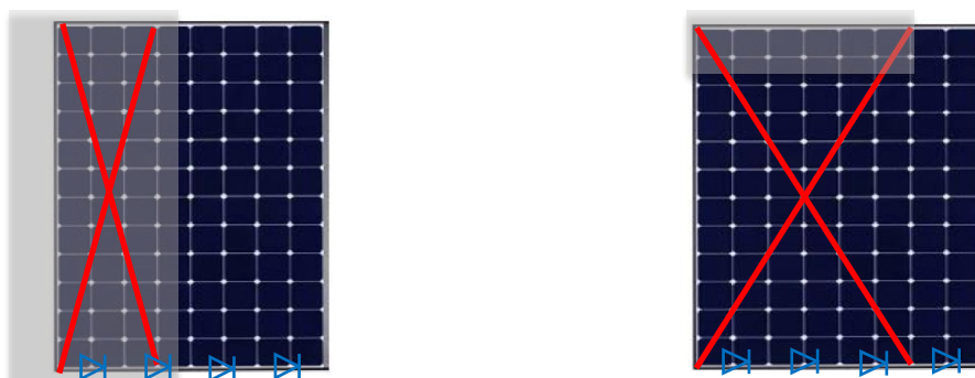
Figure 28 : Impact of a shade according to its position on the photovoltaic panel
