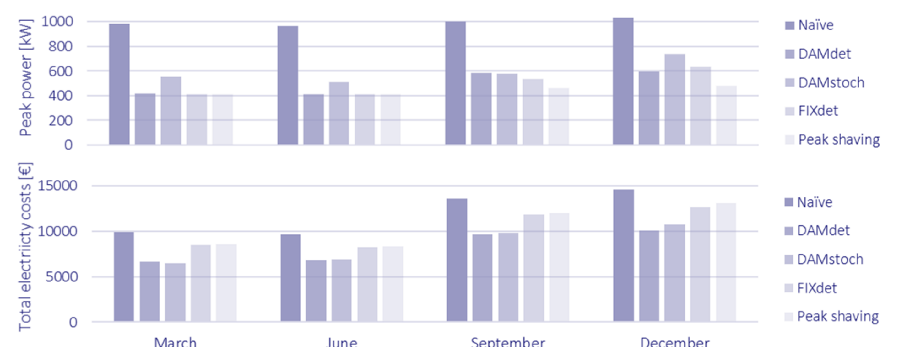
Figure 1. Peak power demand (top), and total electricity costs (bottom) for all charging strategies.
