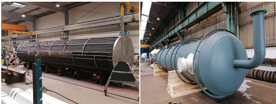
Figure 107 - PCM heat storage integration foreseen within the production plant
