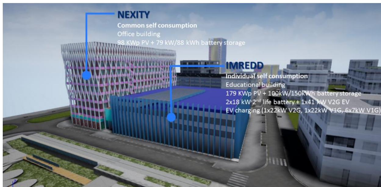
Figure 92 : rendering of the IMREDD and NEXITY case-study buildings for Measure 1 - S 2.1 and 2.3 with relevant technical details (source: UNS/IMREDD - modifications by EDF)
