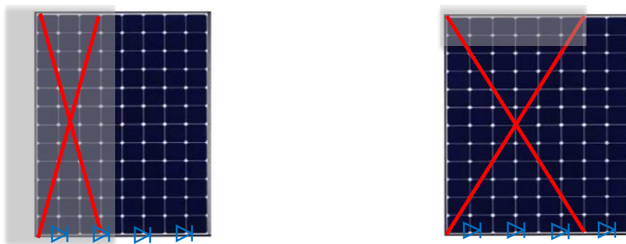
Figure 84 : Impact of a shade according to its position on the photovoltaic panel
