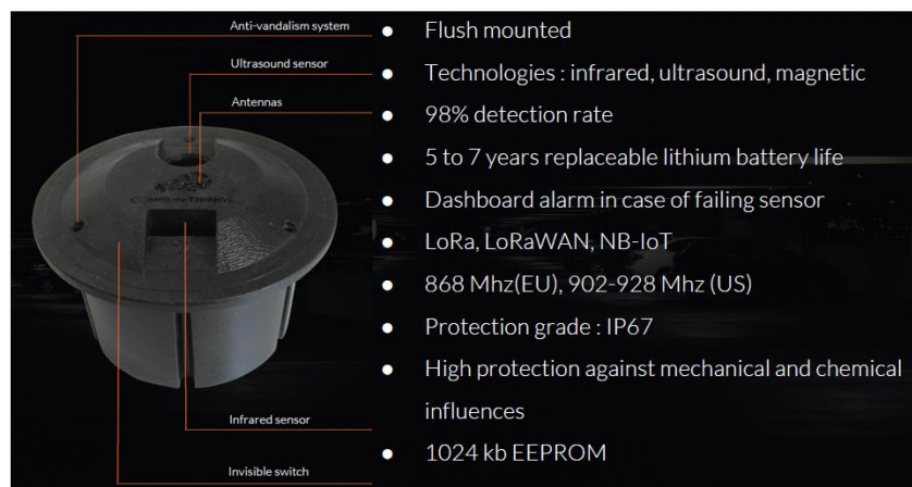
Figure 37: Specifications of the installed parking sensor
