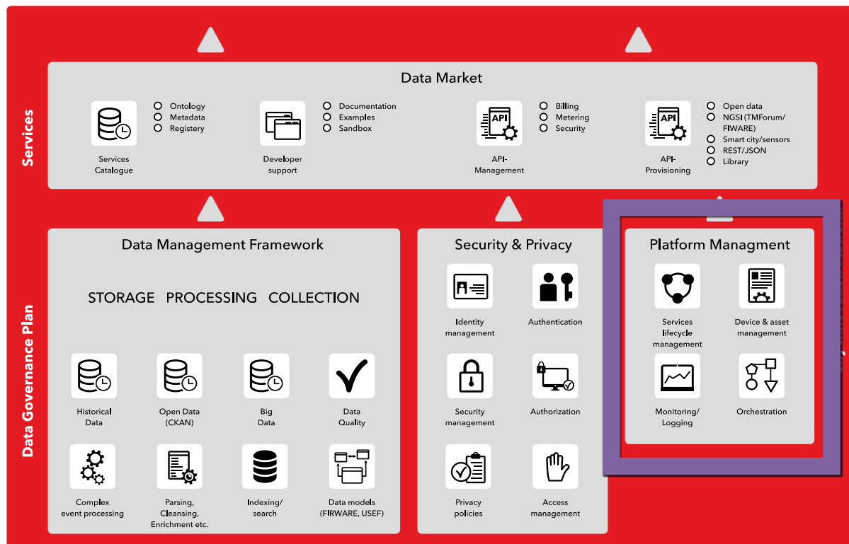
Figure 39 Platform Management component within CIP
